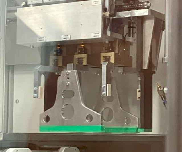
gripper Cell stack for filling in workpiece carrier
